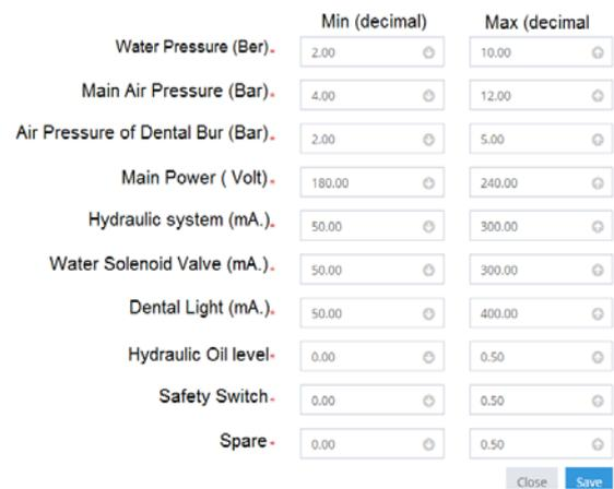
**Figure 6.** Test of data output of the operation control through the online system
