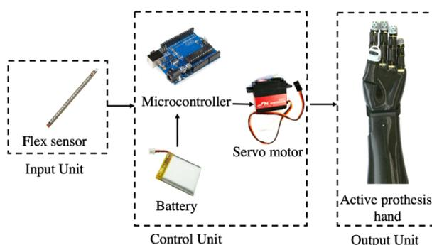
**Figure 1.** Diagram of active prosthetic hand prototype
