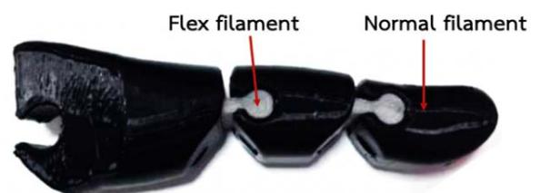
**Figure 9.** Each finger part connected by a connector printed by flex filament
