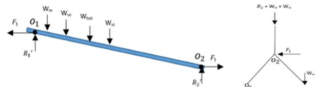
Figure 9. FBD Main structure and Star-wheel mechanism
