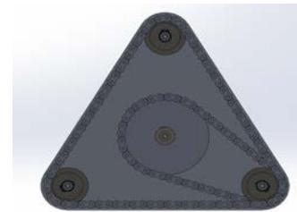
Figure 5. Chain system transmission of the Triple-Delta wheel mechanism
