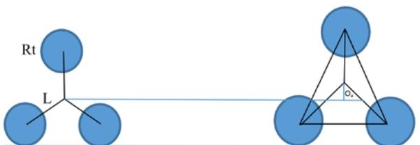
Figure 3. Schematic of structure to join Delta and Star mechanism
