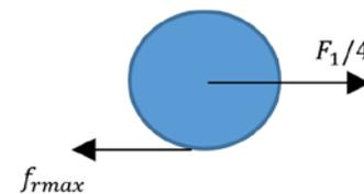
Figure 10. FBD of each frontal wheel in contact with the floor
