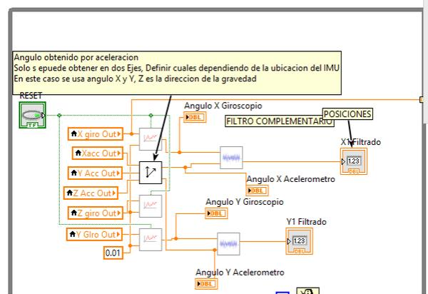
Figure 15. Partial code of the wheelchair control
