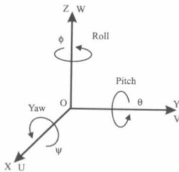
Figure 14. Yaw, pitch and roll angles
