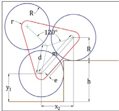
Figure 1. Triple-Delta wheel mechanism parameters
