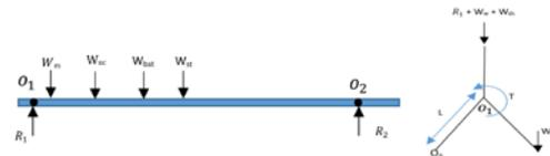
Figure 8. FBD Main structure and Delta-wheel mechanism
