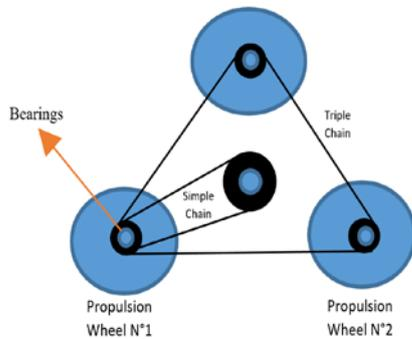
Figure 7. Schematic of the Delta Three-Wheel mechanism
