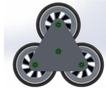
Figure 4. Triple-Delta mechanism
