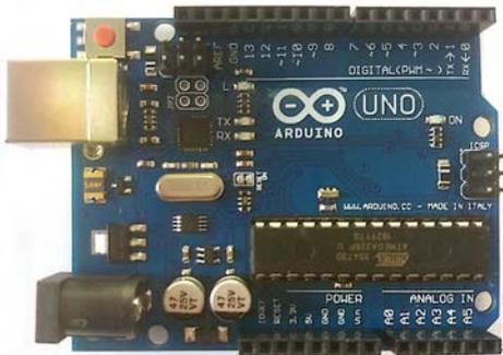
Figure 21. The Arduino UNO R3 board
