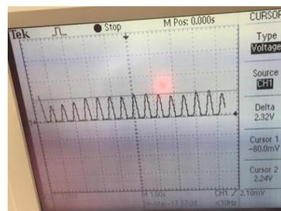
**Figure 10.** The output voltage signal of glucose level at 127 mg/dL
