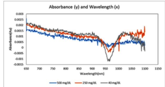
Figure 1. The wavelength absorption of glucose
