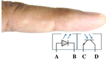
**Figure 4.** Reflective optical sensor principle
