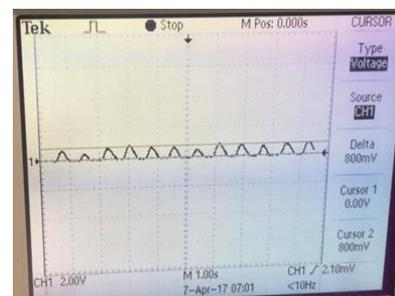
**Figure 9.** The output voltage signal of glucose level at 332 mg/dL
