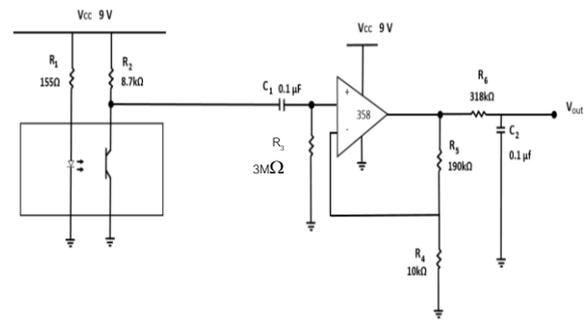
Figure 6. Non-invasive blood glucose sensor circuit
