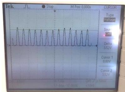
**Figure 11.** The output voltage signal of glucose level at 99 mg/dL
