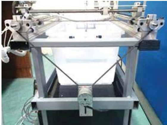
Fig.4:: The gear system on the X axis
