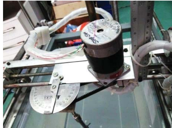
Fig.7:: The gear system on the A axis (clockwise/-counterclockwise (CW/CCW) rotation)
