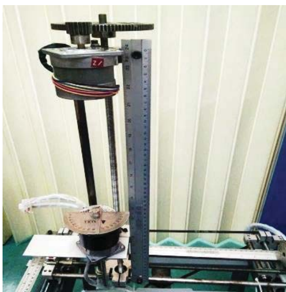
Fig.6:: The gear system on the Z axis
