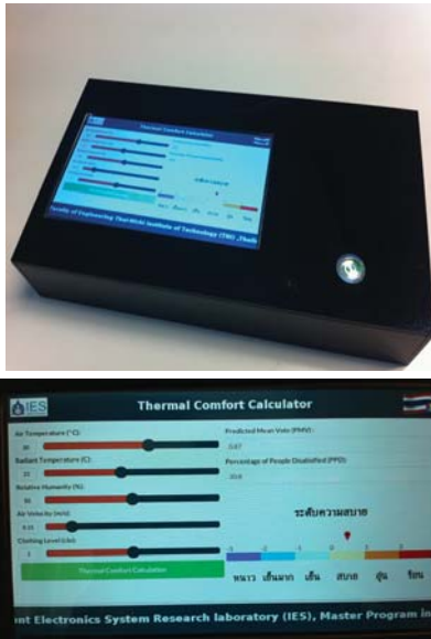
Fig.10: The complete design of the stand-alone PMV calculation device [13].
