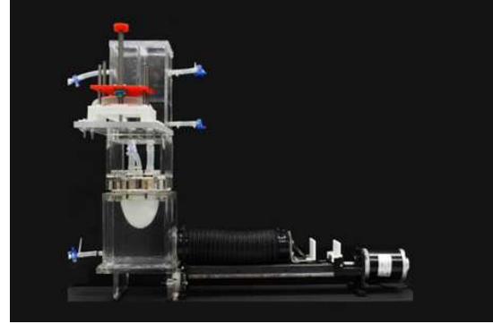
Fig. 3: The completely installation of MCS
