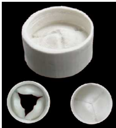
Fig.10:: Structure of AAV (a) while opening (b) and closing (c)
