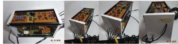
Fig.7:: The EEG hardware prototype set.
