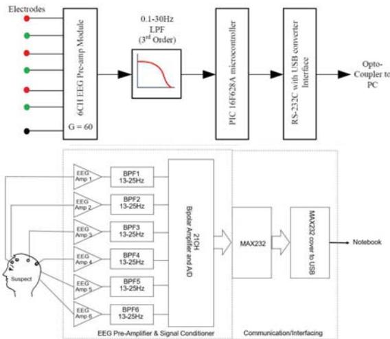
Fig.5:: The design of EEG block diagram.
