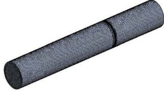
Fig.5: CFD model mesh, isometric view (shore hardness 10A model shown).
