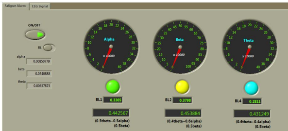
Fig.3: Home-Made Software Interface of the Mental Fatigue Alarm System.
