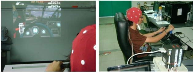
Fig.2: Simulator of for the Fatigue Alarm Experiment.
