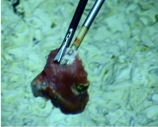
Fig.1: A piece of meat was desiccated by bipolar electro-coagulator (40 W) while grasping forceps were grasping at the side of the bipolar electro-coagulator as a metal guarder.
