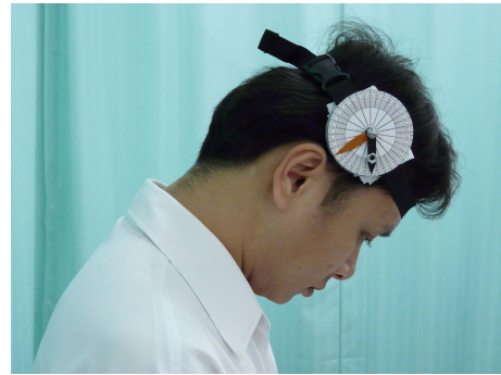
Fig.2: The invented gravitation goniometer with 2-degree scale and 2 sided strap, the figures shows set up of measurement active cervical flexion.)
