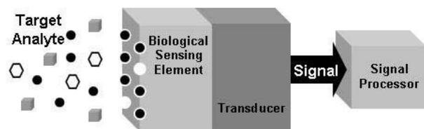
**Fig.1:** Biosensor Configuration
