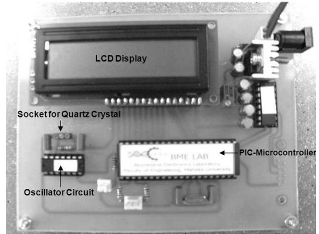
**Fig.3:** Oscillation Frequency Counting Device (In-house developing by Department of Biomedical Engineering, Faculty of Engineering, Mahidol University)
