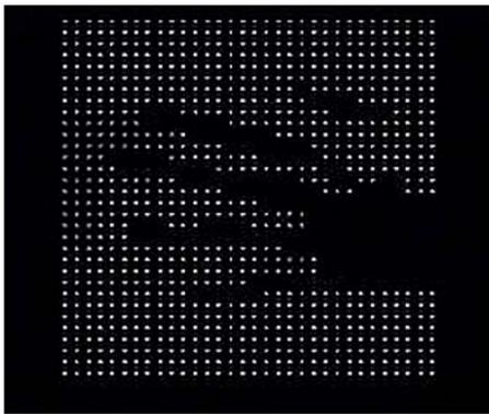
**Fig.5:** Computer simulation of prosthetic vision in the case of  $32 \times 32$  ( $=1024$ ) electrodes.
