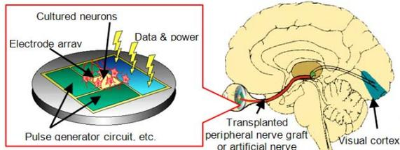
**Fig.1:** Biohybrid visual prosthesis.
