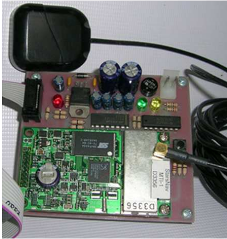
Fig.4: The GPS receiver engine board for transmitting the position of patient
