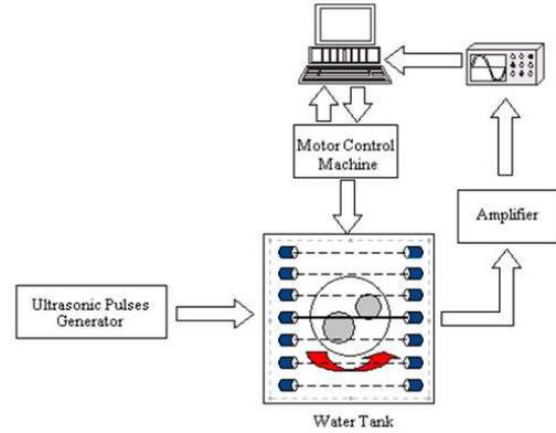
**Fig.2:** Diagram of the acquisition system
