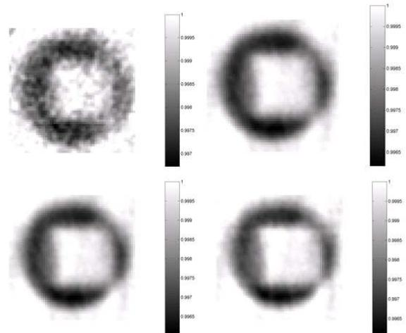
**Fig.9:** Reconstruction of the refractive index of phantom "A" using phase shift at frequency of 1.5 MHz, 3.5 MHz, 3.75 MHz, and 6MHz respectively.
