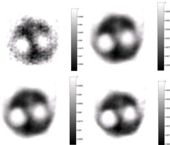
**Fig.10:** Reconstruction of the refractive index of phantom “B” using phase shift at frequency of 1.5 MHz, 3.5 MHz, 3.75 MHz, and 6MHz respectively.
