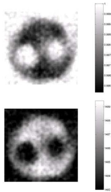
**Fig.8:** Reconstruction of (a) refractive index and (b) sound velocity of phantom "B" using time delay.
