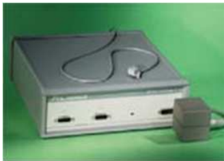
Fig.4: ISOTRAKII TM from POLHEMUS Inc. The precision is 2.4[mm] in position and 0.75[degree] in angle. The area where the positions can be measured is hemisphere whose radius is 76[cm]. The data rate is 30[pts/s] in two receivers case.
