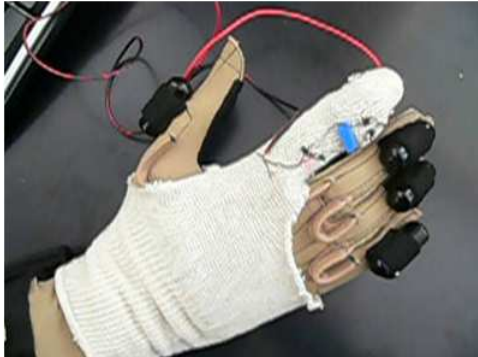
Fig.13: Proto type of a new haptic device using artificial muscle.
