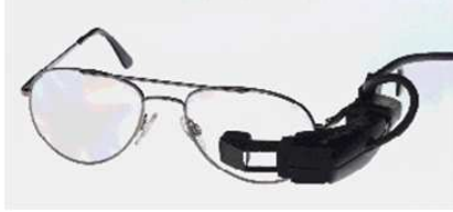
Fig.3: Clip on type micro display. The specifications are VGA ( 640 \times 480 ), 24bits color, refresh rate: 60Hz, view angle: 16[degree] in horizontal and weight: 40g.
